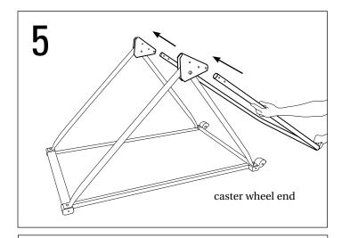
Install screws where indicated. Finger tighten only.
