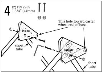
Install nuts to the outside of the floor stand. Finger tighten only.
