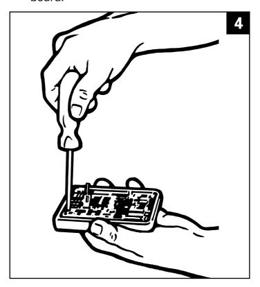
5. Remove and replace rubber key pad (if required). Ensure holes on corners of key pad are in line with locating pins.
