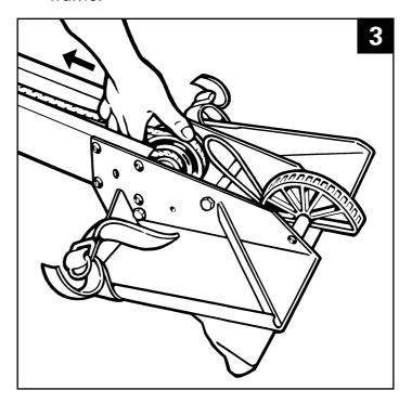
4. Remove frame lock, undo Allen key bolts using the 5/32" Allen key.
